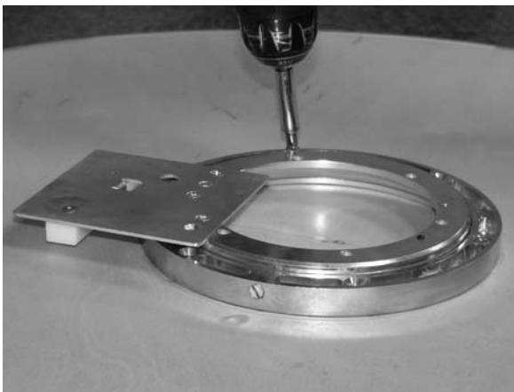
4. Install bearing to tray using (6) of the long screws provided.
